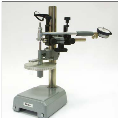
Calibrating a bore gauge.
