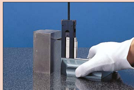
Marking a workpiece using the base, a holder and the scriber point.
