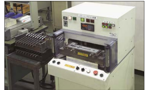
Air leak test equipment for coolant proof caliper.
