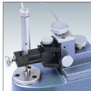
Calibrating a probe head.
