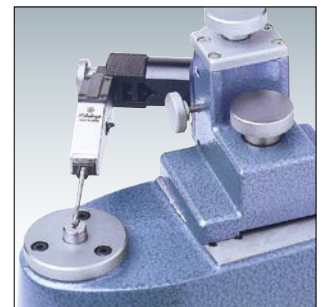
Calibrating a lever probe head.
