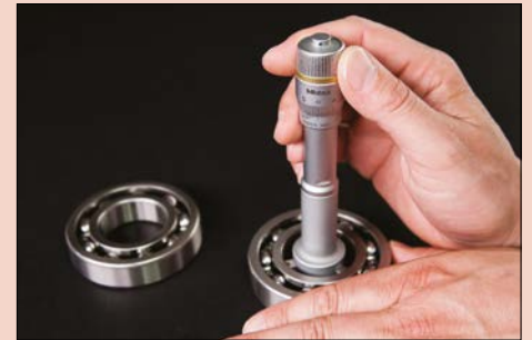
Ball-bearing inner-race inside diameter measurement.
