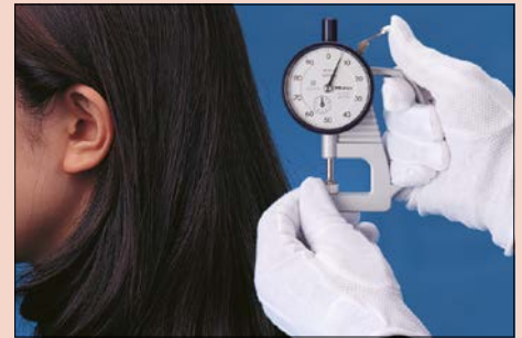
Measuring thickness of a human hair.
