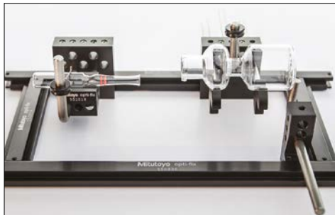
Dissimilar parts located and clamped ready for measurement within the same cycle.
