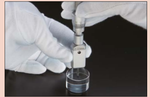
Measuring diameters down to 2 mm with the two-point model.
