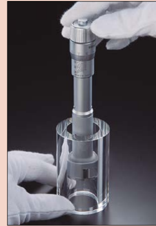
Constant-force device ensures repeatable measurement.
