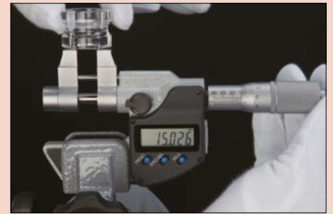
Measuring a small inside diameter.
