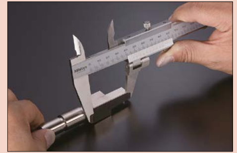
Measuring the distance from a shoulder to the end of a shaft.
