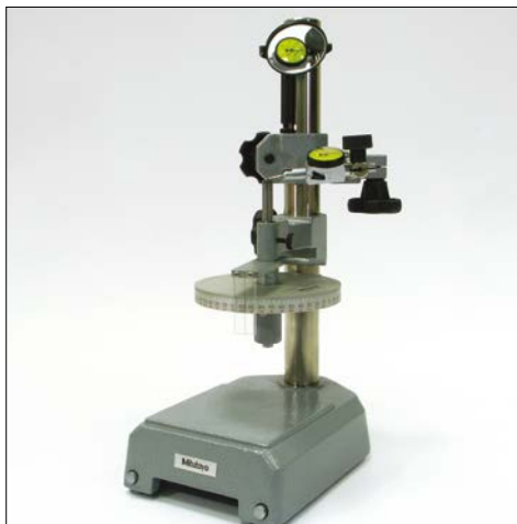
Calibrating a lever indicator.
