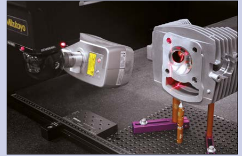
SurfaceMeasure probe scanning a complex surface.
