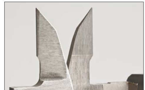
Carbide-tipped jaws for inside measurement.
