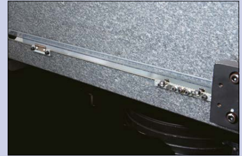
Dust-resistant high-precision glass scales.
