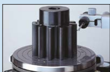
Notched workpiece measurement.
