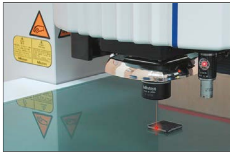
Coaxial laser Tracking Auto Focus (TAF).
